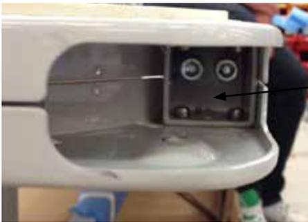
3. When a bumper wheel is removed you can locate two Allen Key side rail screws assembled to the stretcher frame square tubing. **Check that these are tight and fastened.**
