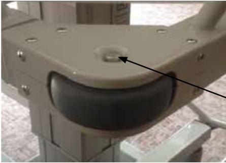
1. Remove the pillow-mattress-drainage hose and break the castors.
